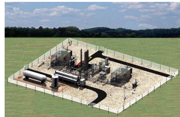
Micro Gas Processing – Well site facility - Rich
