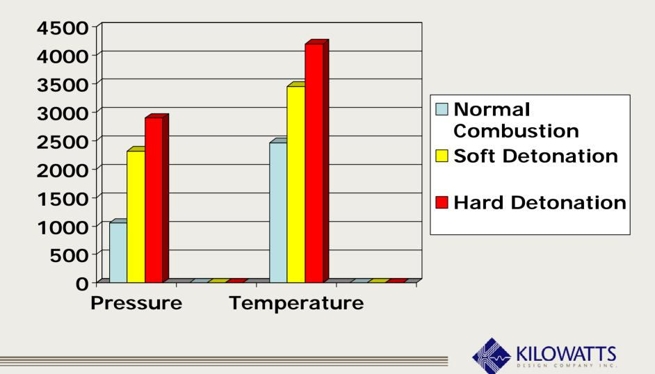
No OEM Combustion Chamber is designed to handle the types of pressures and temperatures that are caused by detonation.
